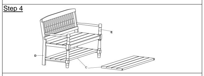
Insert Shelf(C) onto the bottom Rails of Left Leg(D) and Right Leg(E).
