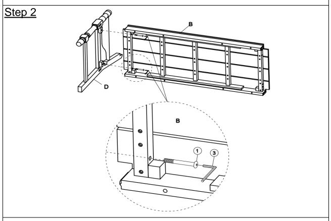
Insert the tenon of the Seat Panel(B) into the mortise of Left Leg(D) and Right Leg(E). Attach Left Leg(D) and Right Leg(E) to Seat Panel(B) using Bolts(1) with Allen Key(3) as shown above.
