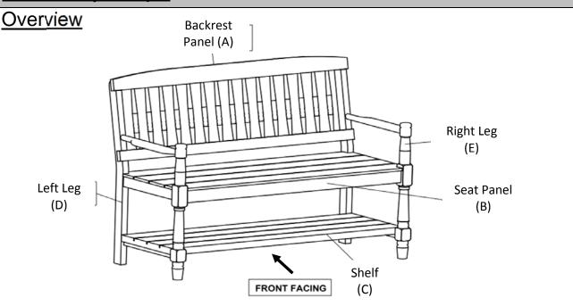
This Bench has multiple parts and may require up to 30 minutes to assemble. To give you an overview of the Bench, the above picture is to help you put the various parts into perspective. Please read through the instructions below to familiarise yourself with the parts and steps before assembly.
