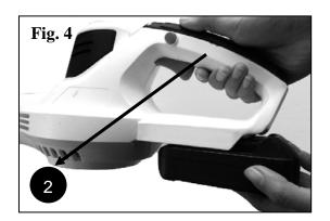
To install the battery pack into the tool, align the rails of the battery pack with the rails in the tool and push the battery into the handle. To connect the battery, slide the battery pack fully forward. Until the latch locks into place.
