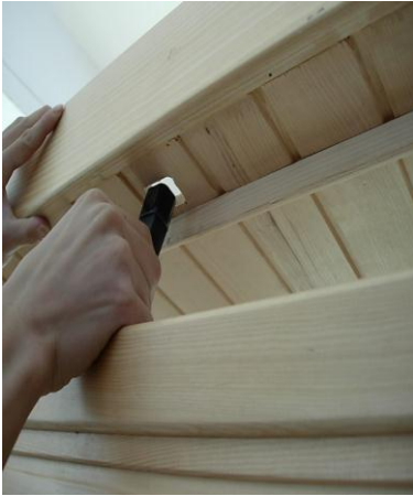
FIG 12 Slip cords/wires through corresponding holes
