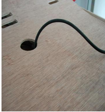
FIG 18 Pull Power Cord through Roof Cover
