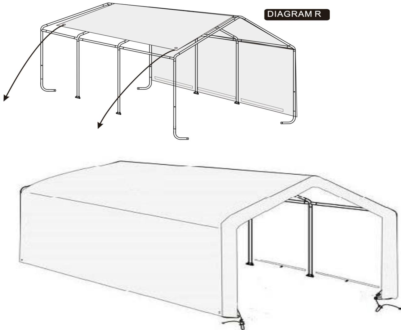
Two people, each positioned approximately one-third into the center of the cover, carefully pull the cover over the frame. When reaching the peak use a step stool or ladder to pass over this height.
