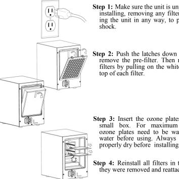
Step 1: Make sure the unit is unplugged before installing, removing any filters or maintaining the unit in any way, to prevent electric
