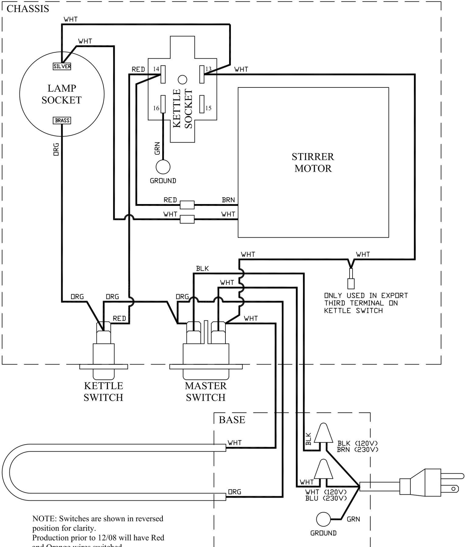
NOTE: Switches are shown in reversed position for clarity. Production prior to 12/08 will have Red and Orange wires switched.
