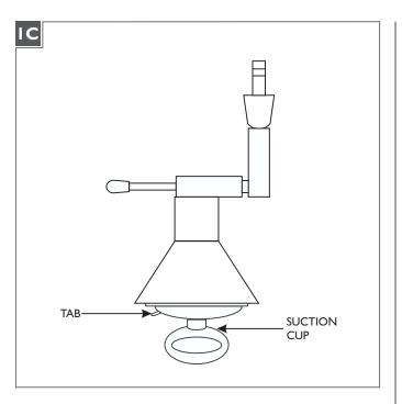
4 Remove the suction cup by pulling on the tab.
