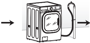
Connecting the drain line
