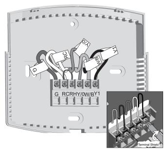
Loosen, but do not remove, the terminal screws.
