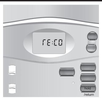
5. Auto recovery – allows heating and cooling systems to gradually recover from an energy-saving setpoint temperature to a comfort setpoint temperature. Auto recovery calculates the time needed to adjust the temperature to the next program setting. When the thermostat is in Auto Recovery mode, the display will flash alternating messages of RECO and the time. Auto Recovery can be disabled by sliding the recovery switch on the back of the circuit board to the disable position.
