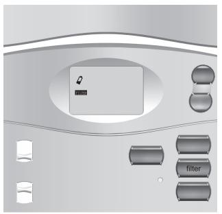
INDIGLO<sup>®</sup> Night-Light - will backlight the display for easy viewing in the dark. Press any button to illuminate the light.
