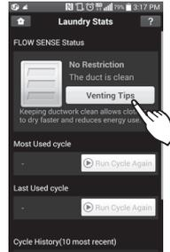
2. If the status shows your home exhaust system is blocked, press the Venting Tips button. Refer to pages 22-23 of this manual for more guidance on venting the dryer. Refer to pages 33-34 of this manual for more information regarding Flow Sense™.
