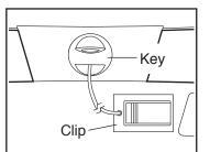
the console. After a moment, the displays will light. IMPORTANT: In an emergency, the key can be pulled from the console, causing the walking belt to slow to a stop. Test the clip by carefully taking a few steps backward; if the key is not pulled from the console, adjust the position of the clip.
