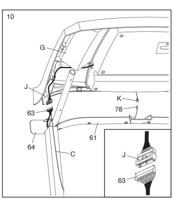
Insert the wires (L) into the Right Handrail (64) through the indicated hole (M) as you set the console assembly (G) on the Left and Right Uprights (66, 76). Make sure that no wires (M, K, 78) are pinched.
