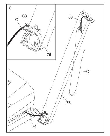
Lay the Right Upright (76) near the Base (74). Press the Upright Grommet (73) into the square hole (D) in the Right Upright. Make sure not to pinch the ground wire (E).
