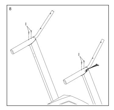
Attach the Console Crossbar (61) to the Left and Right Uprights (66, 76) with four #10 x 3/4" Screws (8) and four #10 Star Washers (23); start all four Screws, and then tighten them.
