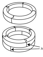
1-Lay out the first course interlocking the blocks making sure that it is level.
