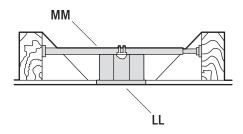
To hang your fan where there is an existing fixture but no ceiling joist, you may need an installation hanger bar (MM) (not included) as shown above.
