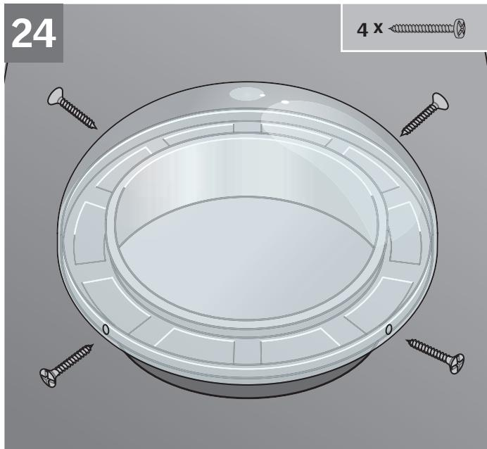
**ENGLISH:** Install and secure the dome with four of the 1" (25 mm) screws provided.
