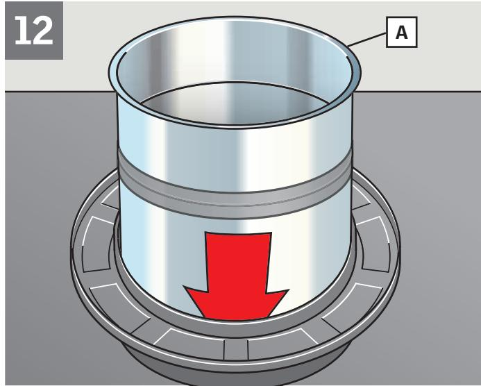
**ENGLISH:** Insert the upper elbow into the flashing allowing the retaining edge **A** to rest on the flashing.
