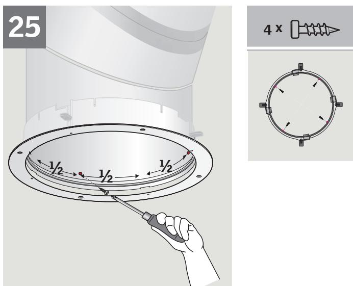
**ENGLISH:** Secure tunnel assembly to ceiling ring with four of the 3/8" (10 mm) screws provided.
