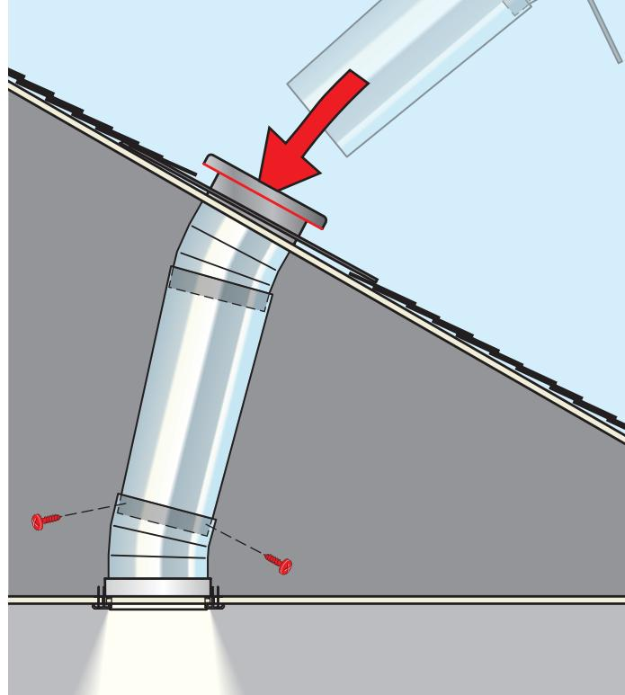
**ENGLISH:** Connect tunnel assembly with the clips supplied. If tunnel section was trimmed or holes do not align, use the screws supplied as necessary.
