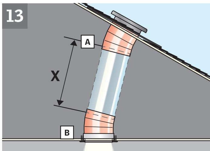
**ENGLISH:** Adjust the angle of both elbows so that they point directly against each other **A**, **B**. Elbows can be damaged if excess force is applied.
