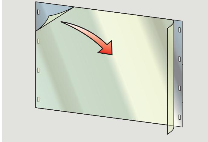
**ENGLISH:** Remove protective film from the rigid tunnel section.
