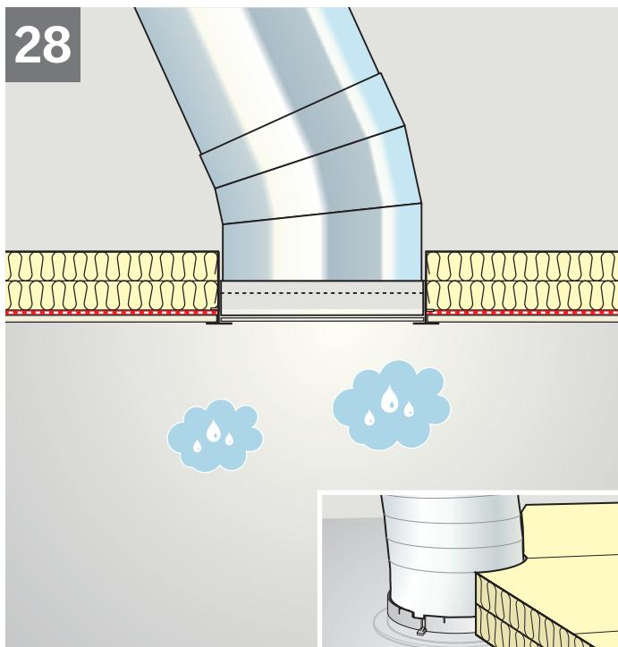
**ENGLISH:** If vapor barrier is installed, insure a tight joint between the ceiling ring and the vapor barrier. Reposition the insulation material around the tunnel.
