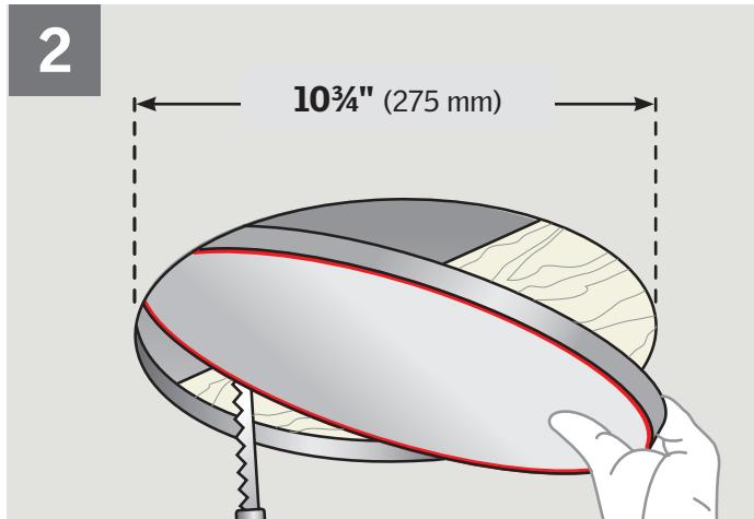
**ENGLISH:** Carefully remove the other parts from the ceiling ring. Rotate trim ring to disengage.
