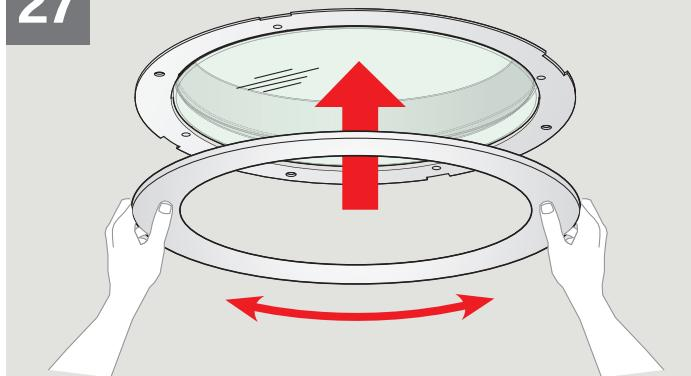
**ENGLISH:** Install the trim ring by aligning notches and rotate to secure.
