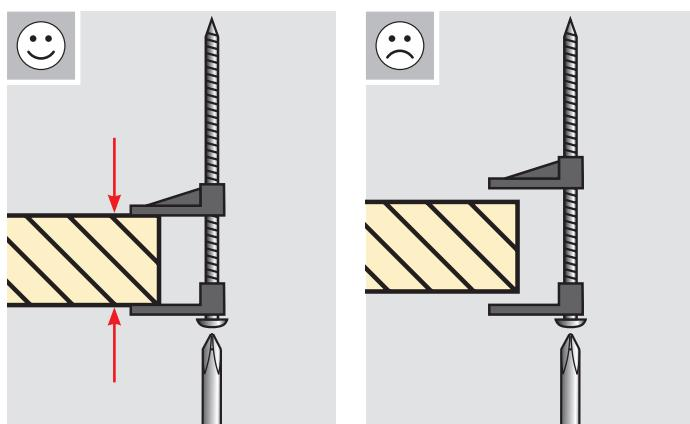
**ENGLISH:** Tip the plastic pins down into hidden position **A**. Insert the ceiling ring. Avoid distortion of the ceiling ring causing the diffuser not to fit smoothly **B**.
