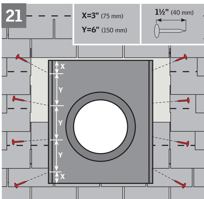
**ENGLISH:** Center the flashing over the rough opening and secure the flange with nails along the sides. Seal all exposed nail heads.
