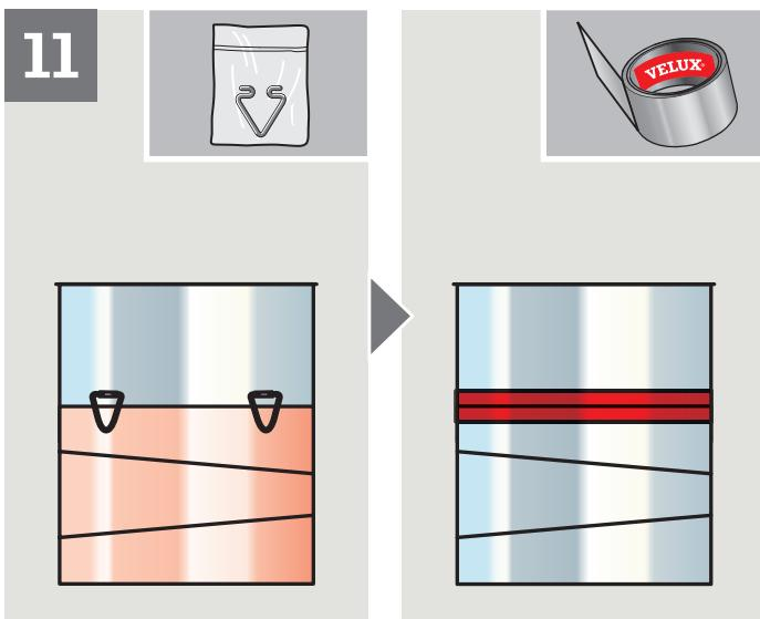
**ENGLISH:** Attach the upper elbow to the top collar. Secure joints with tunnel clips and tape provided.
