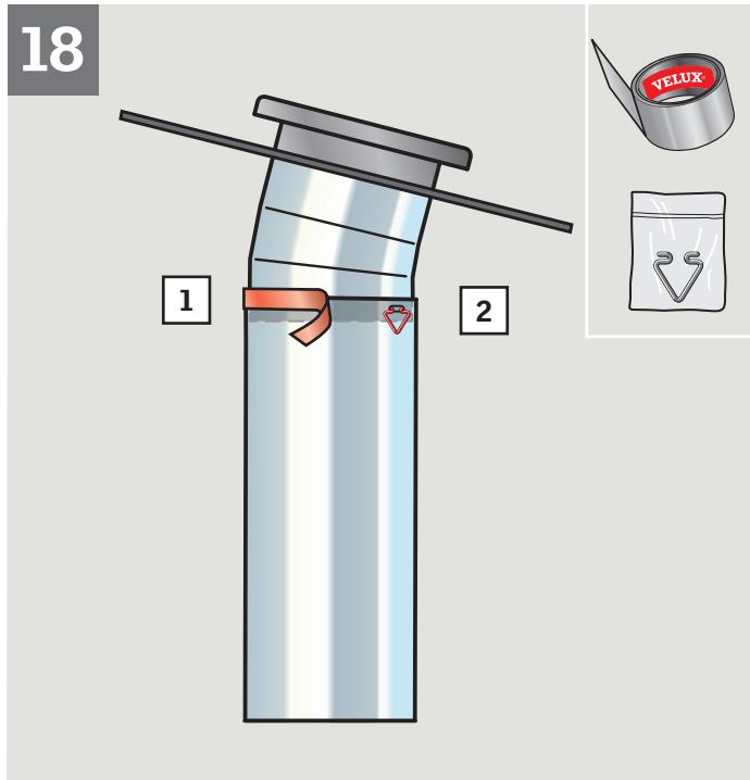
**ENGLISH:** Connect the rigid tunnel section with upper elbow, fitting the rigid tunnel section to go on the outside of the upper elbow. Secure and tape joints with tunnel clips and tape provided **1, 2**.
