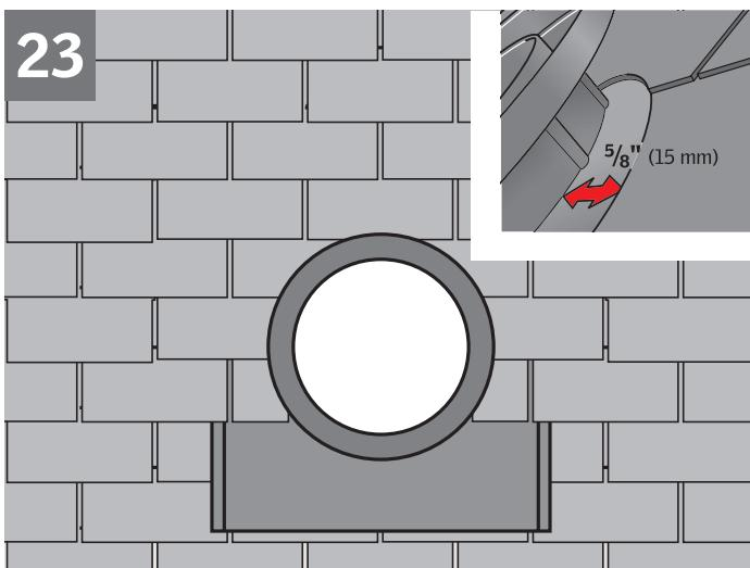
**ENGLISH:** Reinstall roofing material over the flange. Leave a 5/8" (15 mm) channel for water to run off.
