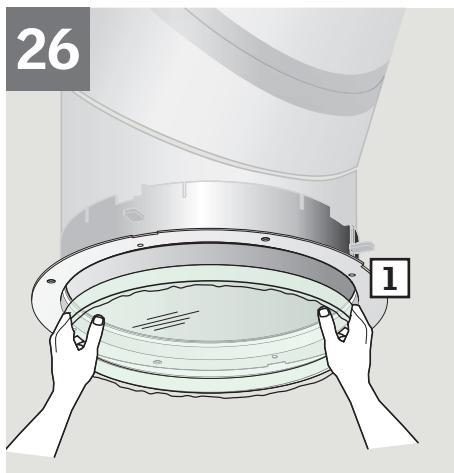
**ENGLISH:** Install the diffuser with the frosted side facing down.
