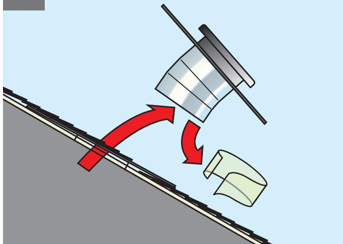
**ENGLISH:** Remove flashing with elbow and remove protective film from upper elbow.
