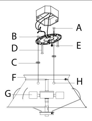
NOTE: Please use the attached hexagonal spanner tool to tighten the center rod until the cables are tight. Then double check that the shade is straight.
