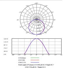
Beam Angle(50%Imax):C0/180Left:57.4 Right:55.3 :C90/270Left:56.6 Right:56.5
