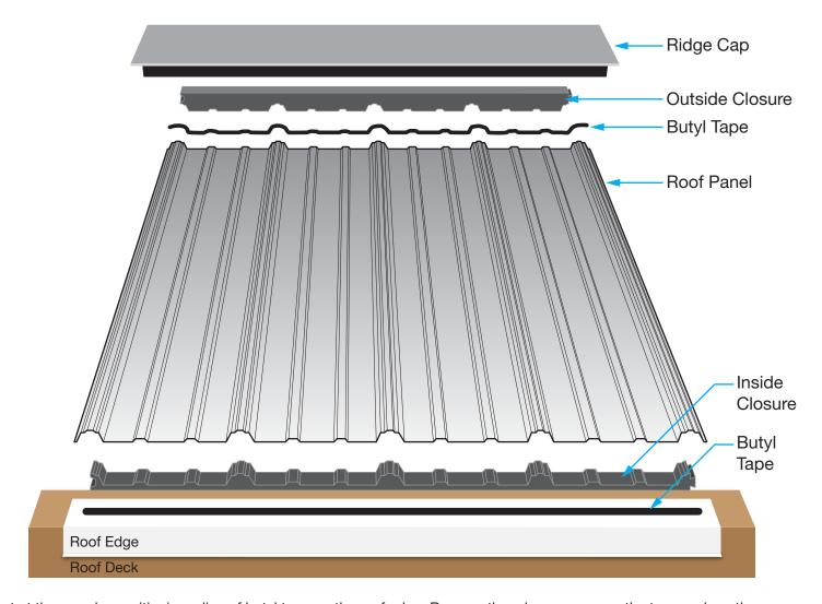
Start at the eave by positioning a line of butyl tape on the roof edge. Remove the release paper on the tape and gently embed the foam closure strip.
