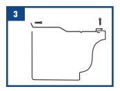
Install the first TITAN 3000 at the beginning of the gutter run by fastening the front edge to the gutter lip using the predrilled hole closest to the end of the TITAN 3000. (Use the 1/2" screws provided. Do not over tighten)
