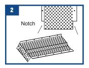
Before installing the first TITAN 3000 measure 2 inches from the end and notch the front and back of the TITAN 3000 Bend remaining 2 inch flap 90 degrees to create an end cap
