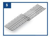
Overlap sections approximately 1 inch and fasten together to the gutter lip
