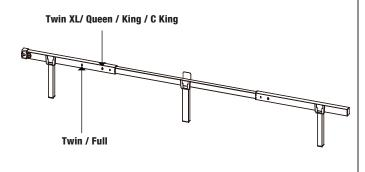
Push the bullet of adjustable leg (B) and pull to adjust size.
