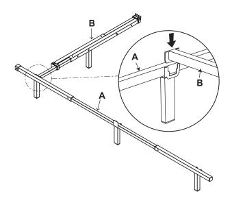
$\hfill\Box$  Insert another two adjustable leg (B) to the adjustable side leg (A).
