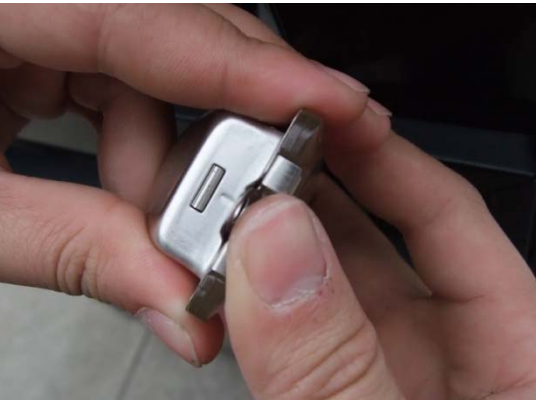
8. Reinstall the bulb case glass onto the bulb case.
