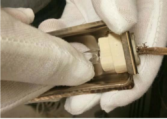
7. Using a glove or cloth, insert new bulb into bulb socket.
