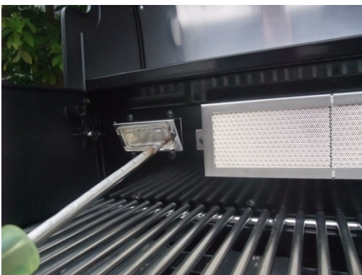
3. Remove the screw and nut holding the bulb case in place.
