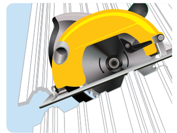
Sawing the panels Figure 4
