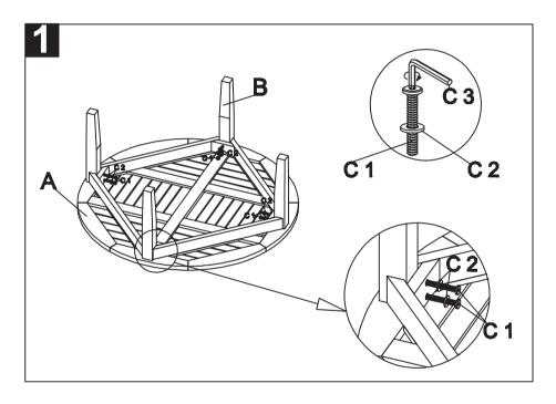
Step 1: attach the leg (B) to the top (A) by using washer (C2) and Allen Bolt (C1) as shown on the picture. Tighten all legs by using the Allen Key (C3).
