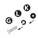
Note: Place the split washer (L) against the head of the machine screw (G) and then add the flat washer (K) before screwing the leg on
