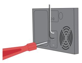
4 Connect one wire from the Power Amp to the "Front" terminal. Connect the other wire to the "Transformer" terminal, leaving the existing doorbell wires in place. Secure both screws before continuing.
