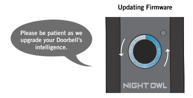
4 When the firmware starts to upgrade, the Status Light turns OFF.
