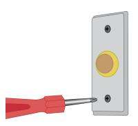
3 Place the Doorbell on the wall or use the provided mounting template to mark the positioning for the new holes.
