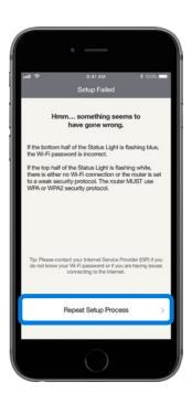
9 If the Doorbell fails to pair, you MUST repeat the "Pairing Process". Select "Repeat the Setup Process" to start the "Pairing Process" again. You may need to set the Doorbell to pairing mode. Press and hold the "Reset Button" as described in Hardware Section.
