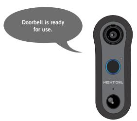
A Doorbell's LED Status Light turns white and spins clockwise (if in Factory Settings or if no Wi-Fi credentials exist) and plays the voice prompt "Doorbell is in Pairing Mode." Doorbell remains in Pairing Mode until it is connected to a Wi-Fi network.
