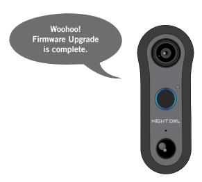
6 If the download was unsuccessful, the Doorbell says, "Oops, Doorbell firmware upgrade failed. Try again later," and the Status Light alternates between a pulsing blue and white. The Doorbell returns to ON/Standby status, and the Status Light turns to solid white (as long as no other status issues are found during "Status Check Process").
