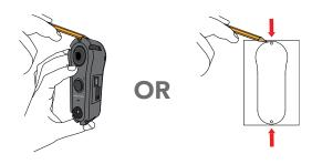
For stucco, brick, or concrete, make the new holes using a 15/64 drill bit and insert the provided plastic anchors into the holes. For wood or siding, use a 3/64 drill bit and save the wall anchors for another project.
