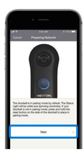
3 When in pairing mode, the Status Light is white and spinning clockwise.
