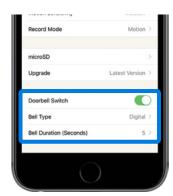
Bell Duration is set to 5 seconds by default and indicates the approximate amount of time the Digital Chime will be active after it is pressed.
