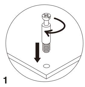
Screw the cam bolt into panel.
