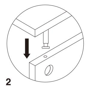
Insert the cam bolt into the bolt hole of joint panel.
