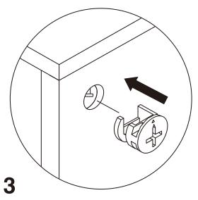
Align the cam lock with its side opening (or arrow) pointing to cam bolt.
