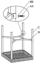
Attaching the connector ring
