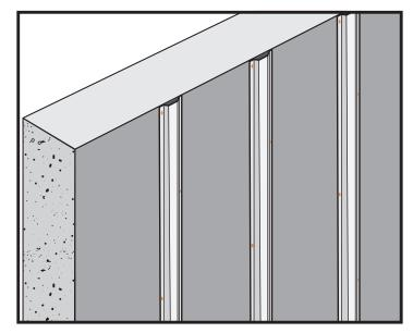
When "furring out" a concrete wall, Furring Channel should be attached vertically with concrete nails or power actuated fasteners.
