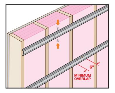
Where Furring Channel needs to be spliced, a minimum 6" overlap is required. The splice is secured with 2 sheet metal screws.
