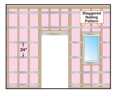
In typical wood frame wall applications Furring Channel is attached perpendicular to framing, with  $#9 \times 1-1/2$  in. screws or 10d nails. Space the channels 16" or 24" O.C.
