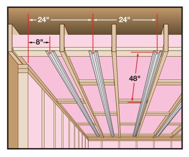
In ceiling applications, furring channels can be attached directly to the underside of the building structure using tie wire, screws or nails.
