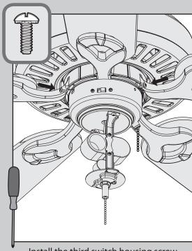
Install the third switch housing screw.
