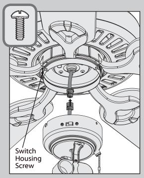
Partially install two of the switch housing screws found in the ≡ hardware bag. Connect the plugs from the upper and lower switch housings. Make sure to line up the colored markings on the connectors.
