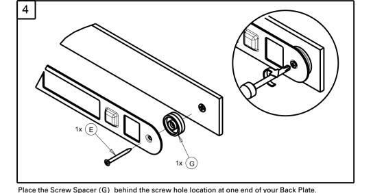
Thread the #6 Screw (E) through the Back Plate and Screw Spacer as shown.
