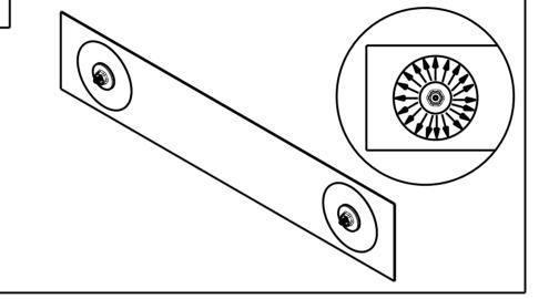
With Thumb Nut and back plate removed, firmly press on IncrediGrip™ pads and smooth the air bubbles out. Work from screw post towards the outer edges of the pads. Optimal performance is achieved with removal of all air pockets from under clear pad area and from behind the mounting post. The failure to remove all air pockets may cause the pads to slip and the basket to fall, causing
