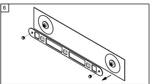
Remove the Thumb Nut and then back plate from the Mounting Pad Assembly
