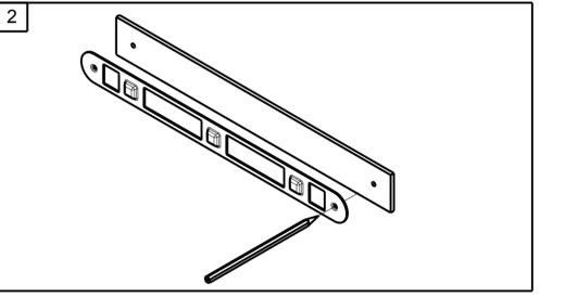
Use a pencil, mark the hole locations at each end of the Back Plate.
