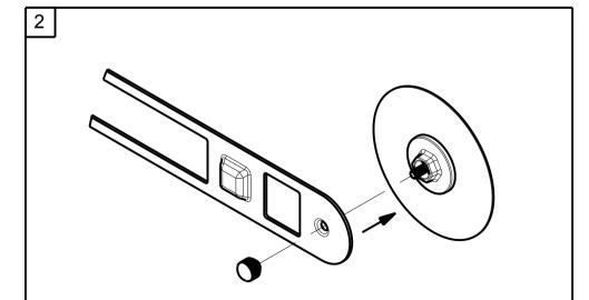
Using the Thumb Nut, attach the IncrediGrip™ pads to the mounting points at each end of the Back Plate as shown. Do not remove the thin protective film on the back of the IncrediGrip™
