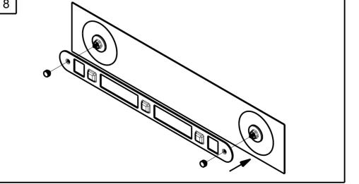
Once the IncrediGrip™ pads have been secured to the mounting surface, refix the back plate onto the Mounting Pad using thumb nut. For optimal performance, wait 30 minutes before loading cup and
