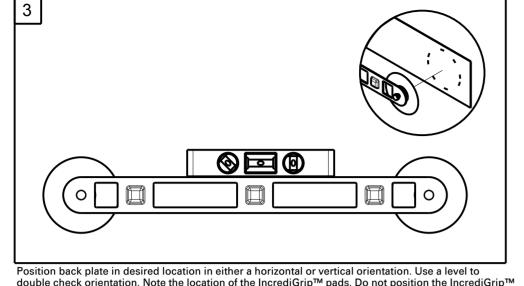
Position back plate in desired location in either a horizontal or vertical orientation. Use a level to double check orientation. Note the location of the IncrediGrip™ pads. Do not position the IncrediGrip™ pads across any tile grout lines or other surface feature that could interfere with application. If one or more of the pads appear to cover a grout line, move IncrediGrip™ pads along back plate to an
