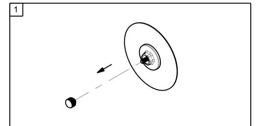
Remove the Thumb Nut from the Mounting Pad Assembly.
