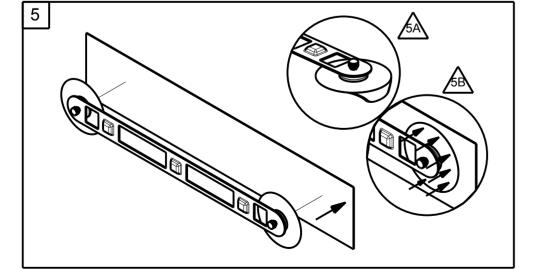
5A) Remove the protective film from the IncrediGrip<sup>™</sup> pads and locate assembly onto mounting surface in desired position. 5B) Using your fingers, partially secure the IncrediGrip<sup>™</sup> pads at each location by pressing the pads firmly into the wall.
