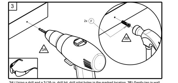
3A) Using a drill and a 3/16-in. drill bit, drill pilot holes in the marked location. 3B) Gently tap in wall
