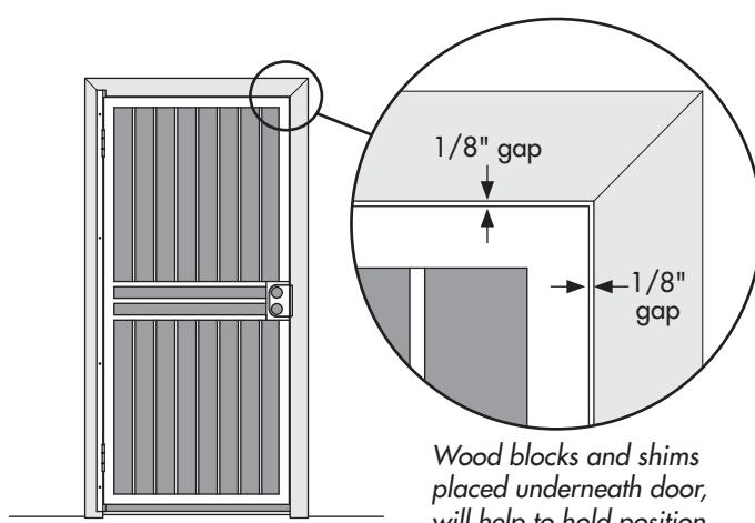
Position door/hinge-side jamb assembly (A) in front of opening. Allow for a 1/8" gap between the lock-side edge of door and inside-edge of your mounting surface, as well as a 1/8" gap between the top-edge of door and bottom-edge of your mounting surface (see illustration).
