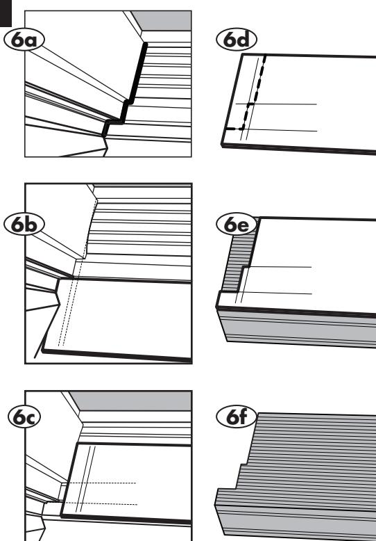
The contour of door framing varies (**6a**) making it necessary to cut the threshold plate (**E**) to fit. We recommend cutting a cardboard template to fit the opening first to avoid incorrectly cutting the threshold plate.
