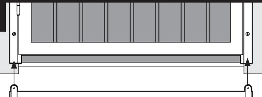
Place bottom bar (**D**) beneath the side jambs. Both ends should reach the outer edge of the side jambs. Hold in place and use 5/32" drill bit to pre-drill holes for mounting screws. Attach bottom bar to each side jamb using the provided screws (**H**).
