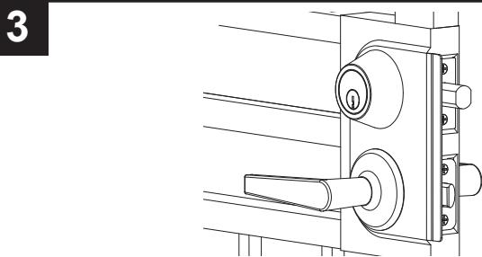
Attach your choice of locksets with 2-3/8" backset. (Sold separately) Fully extend the lock bolts into the "locked" position.
