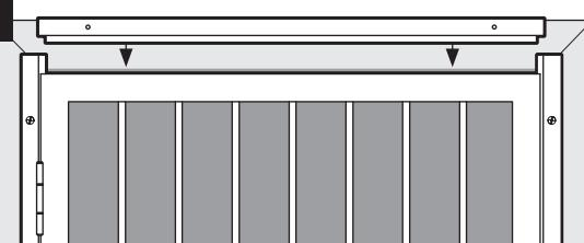
Place the top header jamb (**C**) above the door and between the two side jambs. Spacing should be equal, from left to right, above the door and be similar to spacing determined in **Step 3**. Mark the location of the mounting holes. Set the jamb aside and, where marked, pre-drill 3/16" holes. Return jamb to position and fasten to house using the provided one-way screws (**G**).
