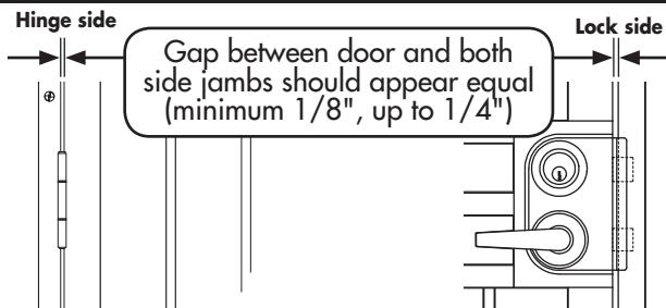
Align the lock holes in the lock-side jamb with the lock bolts extended. Maintain a space between door (**A**) and the lock-side jamb (**B**) equal or similar to the space between the door and hinge-side jamb, from top to bottom. Making sure the lock-side jamb is plumb, mark the location of the mounting holes. Set the jamb aside and, where marked, pre-drill 3/16" holes. Return jamb to position and fasten to house using the provided one-way screws (**G**).
