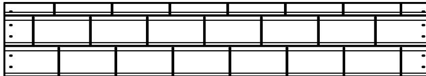
(2) RP1 - PEAK ROOF PANEL - W2A01767 1 3/8"x7 5/8"x44 5/8" (35x195x1134)
