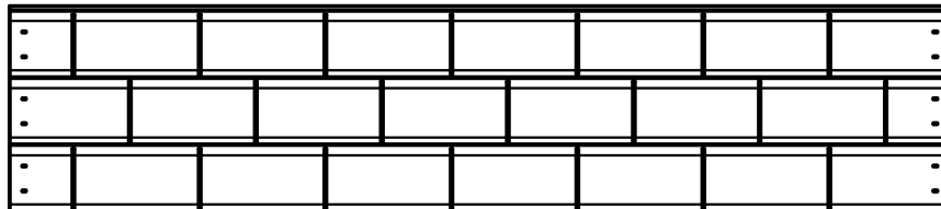
(2) RP2 - MIDDLE ROOF PANEL - W2A01768 1 3/8"x9 3/4"x44 5/8" (35x248x1134)
