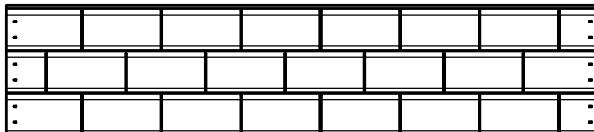
(2) RP3 - LOWER ROOF PANEL - W2A01769 1 3/8"x9 3/4"x44 5/8" (35x248x1134)
