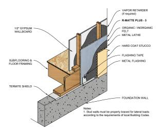
**Re-Siding Construction** - R-Matte Plus-3 may be used in retrofit construction provided the existing siding is sound and solidly attached. It is secured with galvanized nails of sufficient length to penetrate the old sidings, sheathings below and at least one inch into the existing wall studs. Then, cover the R-Matte Plus-3 with a suitable new siding of aluminum, vinvl, fiber cement, wood or wood fiber based products.
