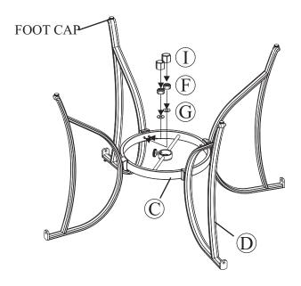
Place the table rim (without glass) upside down on a flat, non-abrasive surface. Attach the table leg to the table rim by using the bolts and washers as shown in Fig.2. Guide the bolts through the holes in the table leg, into the pre-drilled holes in the table rim. **Hand tighten only 2-3 turns.** Repeat for the other three legs.
