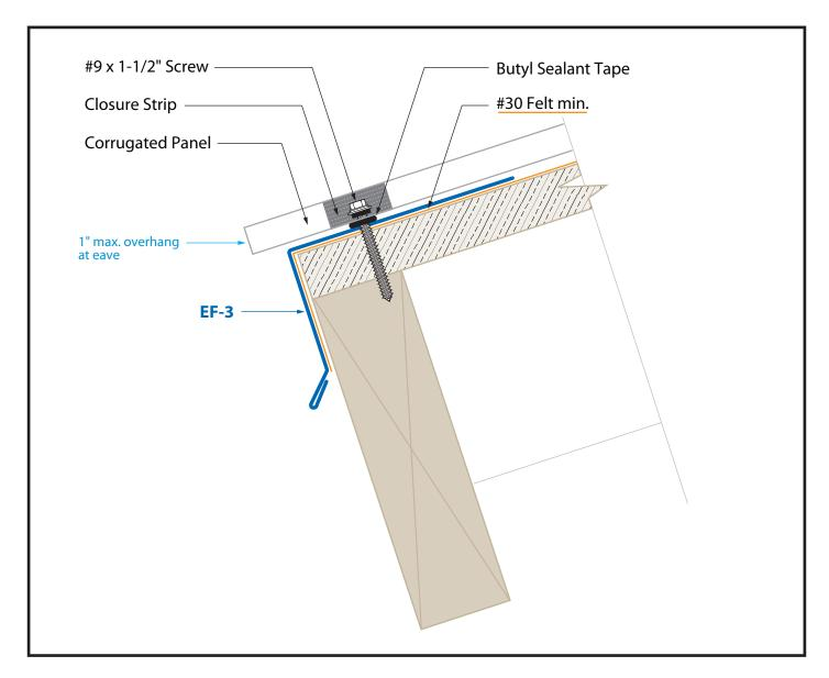
Eave Flashing has **very sharp edges.** Use gloves to prevent injury. This product is not recommended for direct contact with treated lumber.
