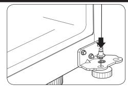
Using a 3/8" socket wrench with a 2-Inch extension and screwdriver, loosen the two bolts and one screw, and remove the Bottom Hinge from right side of the housing.
