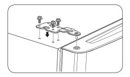
Tighten the bolts. Force-fit Top Hinge Cover over Top Hinge.
