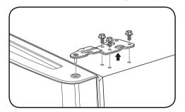
Slightly lift up the refrigerator door and remove it.
