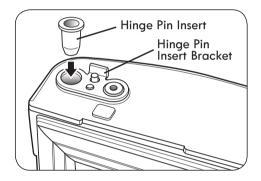
Reverse the Door Closer/Stop by flipping it over. Place it on top of the Hinge Pin Insert Bracket, and tighten both down with the screw.
