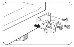
Remove the Decorative Caps on the bottom of the refrigerator housing. You will need these holes for the Bottom Hinge.
