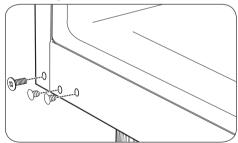
Move the Bottom Hinge to the left side of the housing, keeping the same orientation, and reattach with the two bolts and one screw. The flat screw must be placed on the exterior side of the hinge. Move the Decorative Bolt to the hole on the lower right side of the housing.
