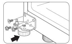
Turn the refrigerator door upside down on a nonscratching surface. Loosen the two screws
