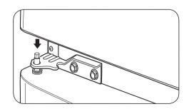
Place the Upper Hinge Pin on top of the freezer door and line up the Upper Hinge with holes on top of the refrigerator. Use the three bolts to replace the Hinge.
