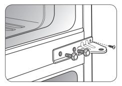
Remove the washer from the Bottom Hinge Pin. Using a ¼" socket wrench, loosen and remove the Hinge Pin from the Bottom Hinge. Reattach the Hinge Pin to the opposite side of the hinge. **NOTE**: This is easier to do while the hinge is still attached.
