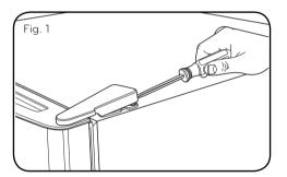
• Using 10 mm or 3/8 inch socket wrench, remove the three bolts and lift the Top Hinge (See Fig. 2). Set parts aside.
