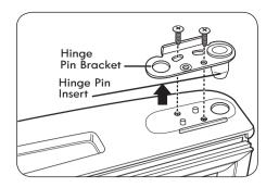
Take out the Hinge Pin Insert and move the Bracket to the other side of the door, keeping the same orientation. Place the Hinge Pin Insert into the left side of the bracket. Tighten the Hinge Pin Bracket to the door.
