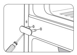
Remove the outer lower Decorative Screw from the housing at the area between the freezer and refrigerator doors. (You will need this hole for the Middle Hinge Bracket.)
