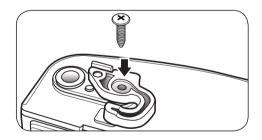
Pry off the cover on the top left side of the refrigerator to uncover the screw holes.
