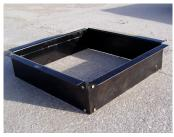
**Step 5**: Assemble the steel insert. Place the 4 sides of the insert on the ground and using 8 bolts provided, bolt the 4 sides of the insert together. Set the steel insert onto the caps as shown. Then place approximately 2" of clean porous rock or gravel inside the fire pit.
