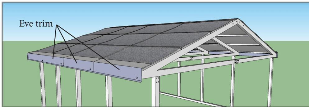
**Step 1** - Begin installing the first Eve trim at the back of canopy frame working forward. Place trim on top of Insulation and end of rafter with drip edge down. Extend it past outside of rafter face  $1\frac{1}{4}$ " (photo 20) and (fig 8 on page 14).
