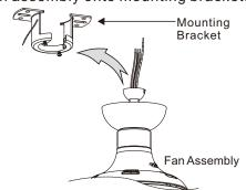
Rotate fan so that the groove on the ball engages the ridge in the mounting bracket.
