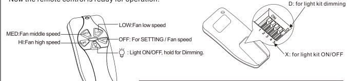
**Note:** The optional Light Kit for this model uses a Dimmable LED Array so the switch should be left at D position.
