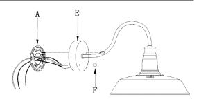
Attach the mounting plate assembly(A) to outlet box with mounting screws (C).
