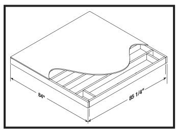
Secure shed to wood platform using 1/4" x 3" lag screws.
