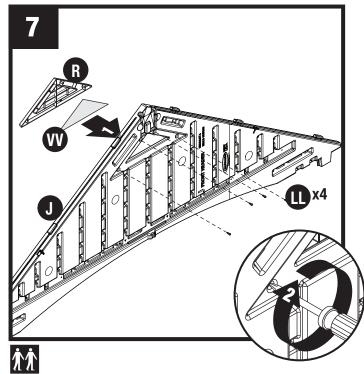
Place fiberglass vent screen (VV) and header vent (R) into front opening in front header (J). Secure through back of header with four screws (LL). **DO NOT** over tighten screws.
