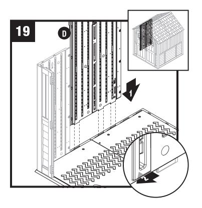
Align tabs on bottom of side panel (D) with slots along front and rear floors. Lower panel into slots and lock in place by sliding panel toward front corner.
