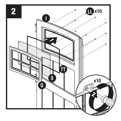
Stand left door (I) vertically. In this order, layer into door channel the window gasket (TT), door window (S), and door window frame (Q). Through the back of door, secure layers with ten screws (LL). Start with four corner screws and finish with remaining screws. **DO NOT** over tighten screws.
