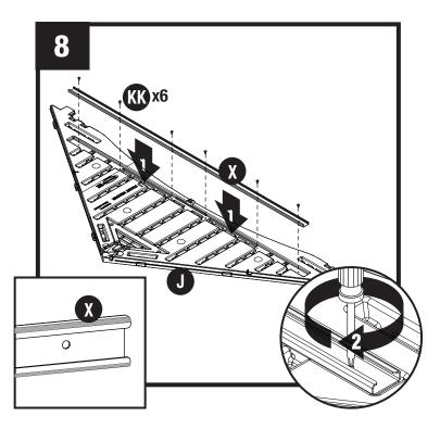
Lay header (J) on ground with lettering side facing up. Place one header beam (X) into pocket on inside of front header (J). Attach with six screws (KK). **DO NOT** over tighten screws.
