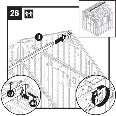
Raise ridge beam (U) up and into rear roof ridge beam bracket. Secure with one 2" hex head cap screw (HH) and one nut (JJ).
