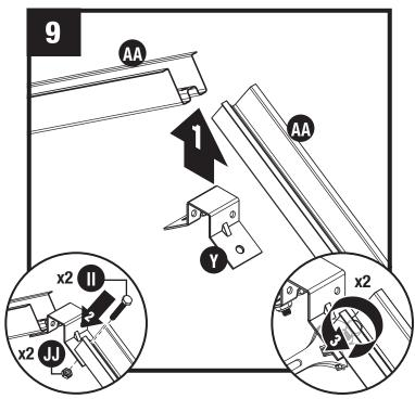
Attach truss bracket (Y) to end of one truss leg (AA) with 1" hex head cap screw (II) and nut (JJ).
