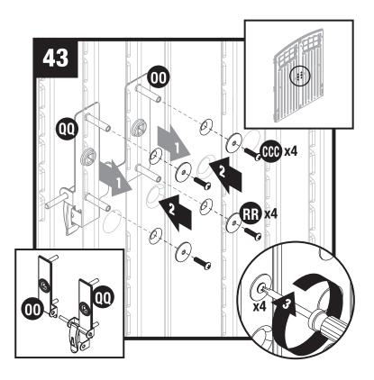
Insert screw stems, on left and right handle plates (OO) and (QQ), through the pre-drilled holes in doors. While holding plates in place on exterior of door, secure each with two washers (RR) and two machine screws (CCC).
