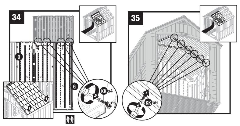
Pull down each lower corner of roof from outside. From inside shed, attach tabs on panel (D) and right front (G) corner to roof panel with four screws (KK).
