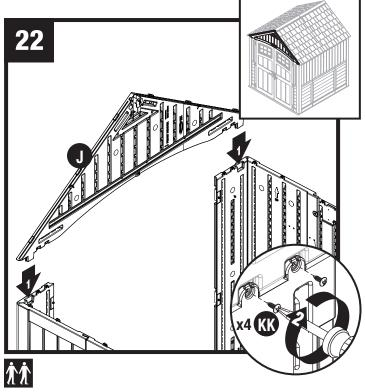
Place front header (J) over door opening and fit two protruding support legs into pockets molded in front corners. Secure front header using two screws (KK) in each front corner.
