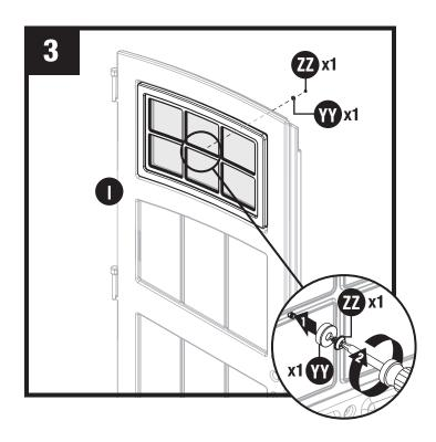
Secure center of window with one washer head screw (ZZ) and sealing washer (YY). **DO NOT** over tighten screws. Repeat on Steps 1-3 for right door (H).
