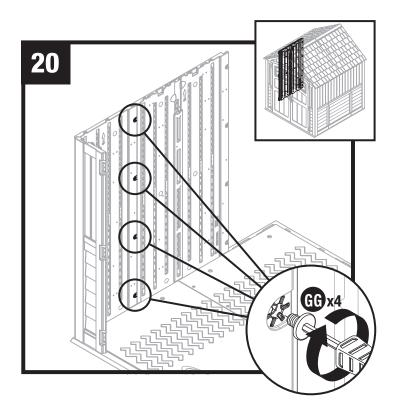
Secure side panel with four easy bolts (GG), working from floor to roof. **DO NOT** use torque wrench. Use easy bolt easy driver (XX) and hand tighten. Easy bolt head will be flush when fully seated. **DO NOT** over tighten easy bolts.
