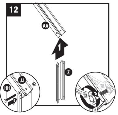
Place window truss tie down (Z) at end of right truss leg (AA). Secure truss tie down with one 2" hex head cap screw (HH) and one nut (JJ).
