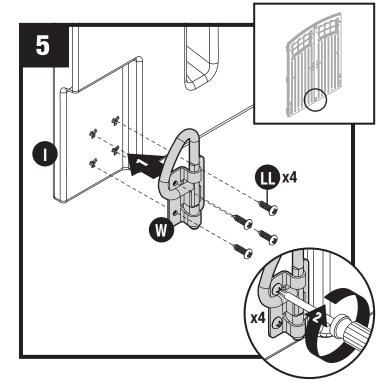
At bottom interior side of left door (I), attach D-ring slide bolt (W) with four screws (LL) through provided holes.
