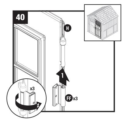
Stand right door (H) upright with three hinge mounts facing right. Slide one metal hinge plate (FF) up onto each hinge mount. Rotate hinge plates to outside of door. Snap metal hinge plate into place by pushing towards door.
