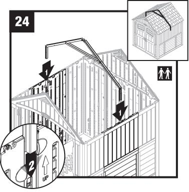
Slide truss assembly into place.
