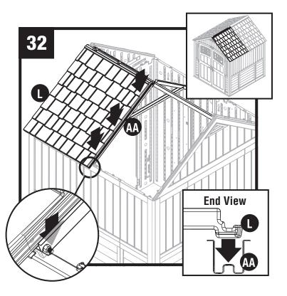
Press edge of right roof (L) into channel on truss leg (AA).
