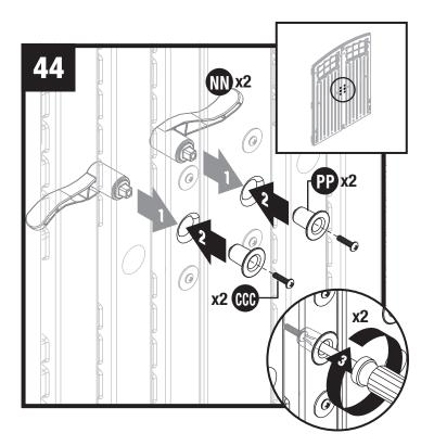
From the outside of doors, insert door handles (NN) through handle plate holes. On inside of doors, place spacers (PP) on each door handle, and secure each with one machine screw (CCC).
