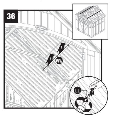
Raise roof support (WW) into position against roof. Slide roof support (WW) into front header. Secure roof support (WW) to underside of truss leg with one screw (LL).
