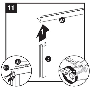
Place side adaptor bracket (Z) at end of left truss leg (AA). Secure adaptor bracket with one 2" hex head cap screw (HH) and one nut (JJ).
