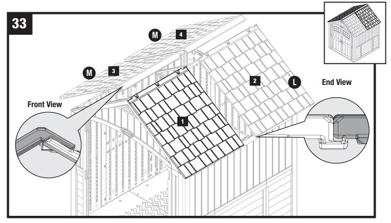
Repeat steps 30-32 for remaining roof panels. Install panels in the order shown.
