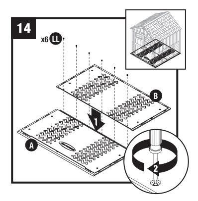
Push front floor (A) and rear floor (B) panels together and secure with six screws (LL).
