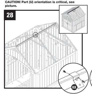
Attach the roof truss assembly to the ridge beam with two screws (KK).
