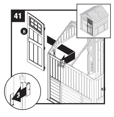
Rotate metal hinge plates to open position. Slide one metal hinge plate over each hinge receptacle on inside of right front panel.
