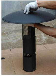
Thread the 3 screws through the tabs into the deflector disk. Then attach the long section of stove pipe to the completed screened section. Place the top stack onto the heater assembly.
