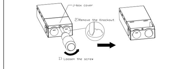
**To remove knockouts:** (Choose one of the four knockouts for the 120V supply connection) Place standard screwdriver on edge of circle and gently strike with hammer. Grip edge with pliers and flex back and forth until removed. (See Fig. 2)
