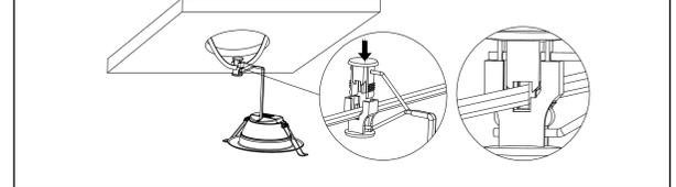
6. Flip up and squeeze the spring-loaded clips above the fixture (see Fig. 6) and insert the fixture into the hole. When the clips reach the hole edge, slowly release them and push up the fixture until both clips flip down onto the ceiling surface. (See Fig. 6)
