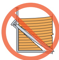
Nail too long
