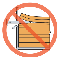
Nail at wrong angle
