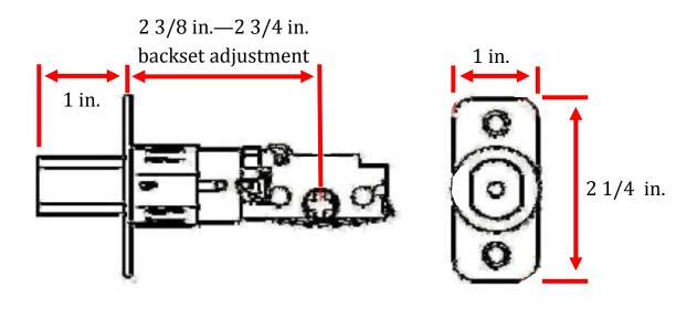
Can be adapted for radius-corner, square-corner or circular drive-in applications
