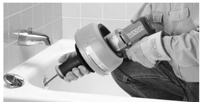
Figure 9 – Push Cable Down Drain Line
