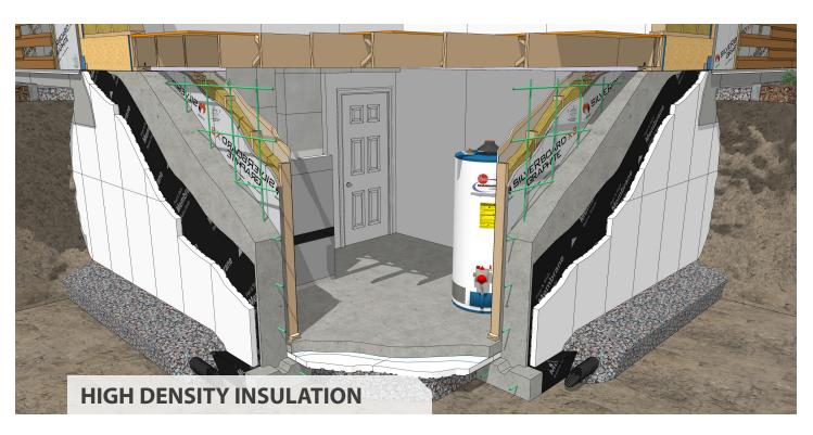
Amvic's multipurpose rigid insulation is a Do-It-yourself (DIY) molded panel using closed cell Expanded Polystyrene (EPS) with one flat face. The second face of the panel has bi-directional channels that can be used as either venting or water drainage, depending on the application.
