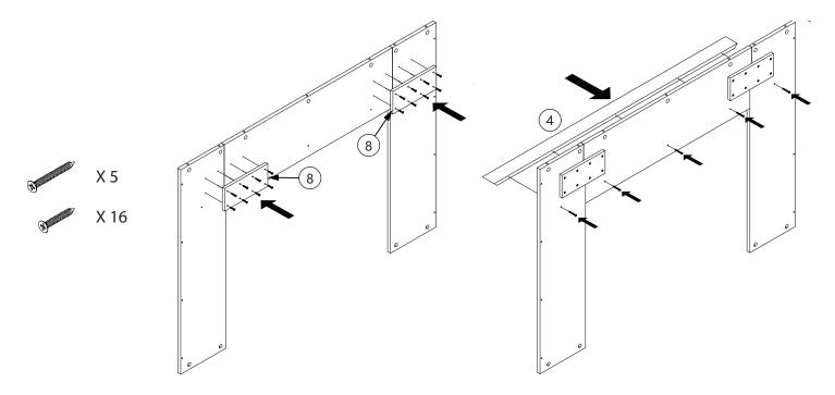
3. Attach the (#6) Left Side and (#7) Right Side Panels using eight Cam Locks (A) and eight Cam Bolts (B) as shown.
