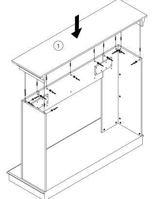
5. Attach the (#1) Top Mantel by using eleven Cam Locks (A) and eleven Cam Bolts (B) as shown.
