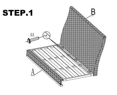
Please connect A and B with AA. The screws have to be screwed in halfway, not to the end.
