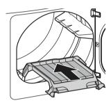
Make sure it is seated evenly on the edge 2 of the inner door rim and resting flat on the inside of the dryer.
