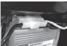
CONNECT AND POSITION BATTERY WIRES AS SHOWN BEFORE INSTALLING FRONT COVER PLATE
